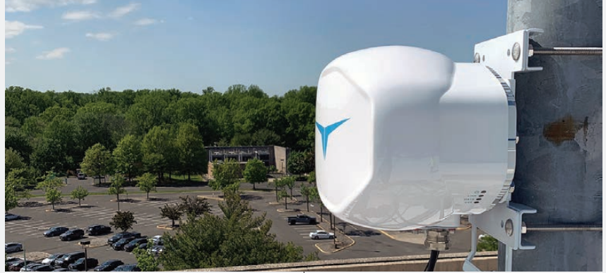
Transcelestial's optical ground stations [left] are small enough to fit on a building's rooftop, such as this one in Singapore. Transcelestial's space-to-ground laser technology is informed by the company's previous work developing terrestrial optical networks.
