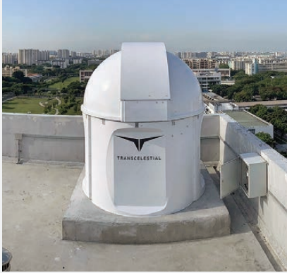
Transcelestial's optical ground stations [left] are small enough to fit on a building's rooftop, such as this one in Singapore. Transcelestial's space-to-ground laser technology is informed by the company's previous work developing terrestrial optical networks.
